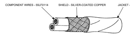
JACKET - ULTRA LOW FLUORIDE, RADIATION-CROSSLINKED, MODIFIED ETFE
