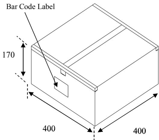
5 reels at maximum shall be packed in a outer package.
