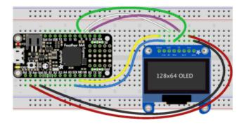
Microcontroller 3V to OLED Vin
