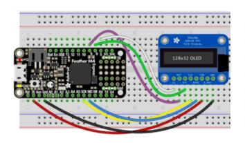
Microcontroller 3V to OLED VIN
