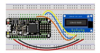
Microcontroller 3V to OLED VIN
