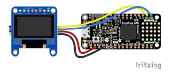
You do not need to alter the jumpers on the back - I2C is the default configuration on this display!
