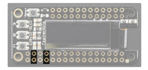
OLED displays do not have a backlight, and are fairly low power, this display will draw about 10mA when in use. The display uses 3V power and logic so we just connect to the 3V and GND pins from the feather, as indicated above.
