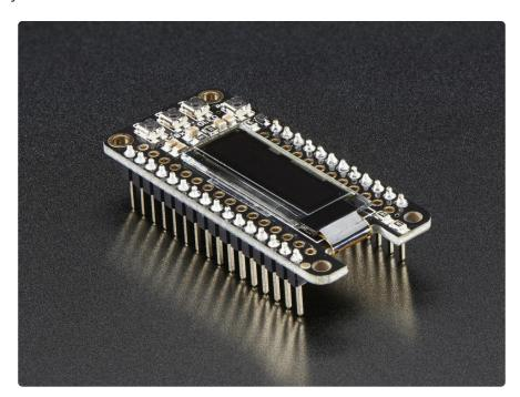
Tested works with all of our Feather boards. The OLED uses only the two I2C pins on the Feather, and you can pretty much stack it with any other FeatherWing, even ones that use I2C since that is a shared bus.
