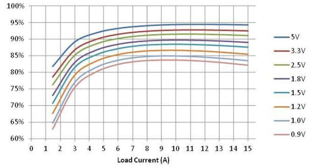
Figure 2. Efficiency vs. Load.  $V_{in}=12V$ ,  $F_{sw}=500kHz$
