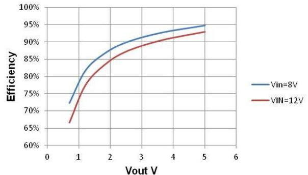
Figure 6. Efficiency vs. Output Voltage,  $I_{out}=15A$ ,  $F_{sw}=1MHz$
