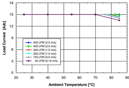
Figure 9. Thermal Derating Curves. Vin=12V, Vout=5.0V, Fsw=500kHz
