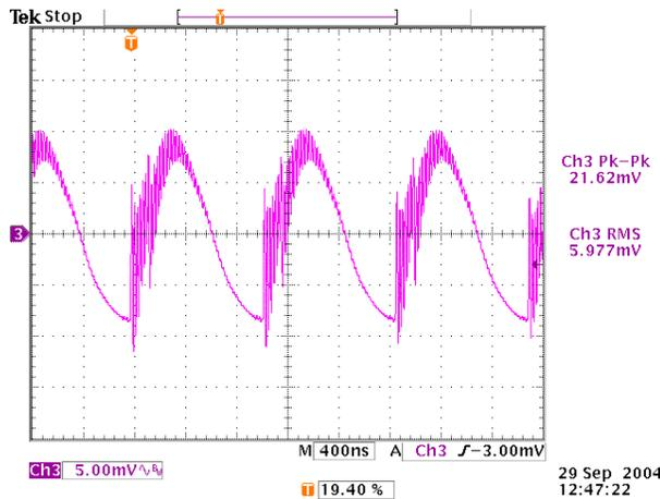
Figure 44. Output Voltage Noise, Full Load, No Interleave
