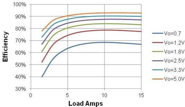
Figure 5. Efficiency vs. Load.  $V_{in}=12V$ ,  $F_{sw}=1MHz$
