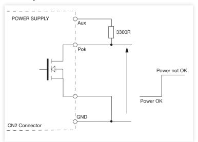
Open drain signal, low when PSU turns on. Maximum sink current: 20mA Maximum drain voltage: 40V
