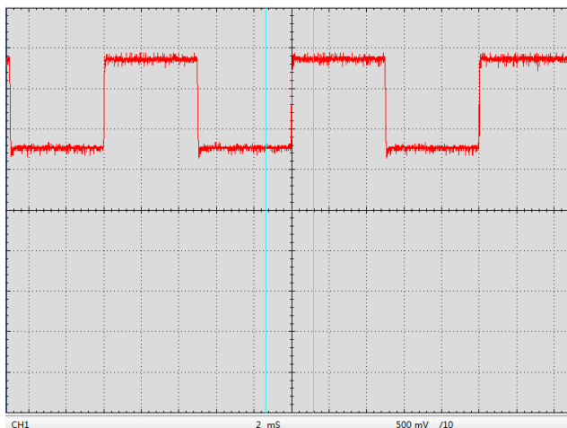
Figure 8. Digital Modulation Response at LDA Pin
