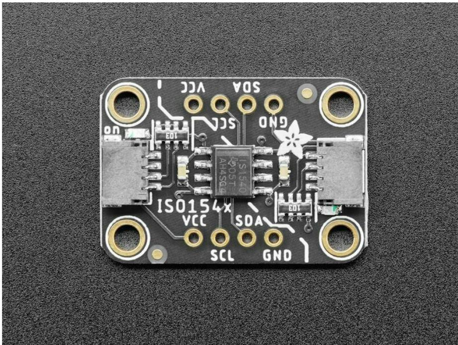
Sometimes you'll find yourself with an I2C bus controller on one side, and an I2C bus device on the other and [you gotta keep em \(electrically\) separated](https://adafruit.it/QsD) (https://adafruit.it/QsD). Maybe because one is Earth-grounded, maybe because you've got some funky power monitoring setup, maybe you want to reduce noise.
