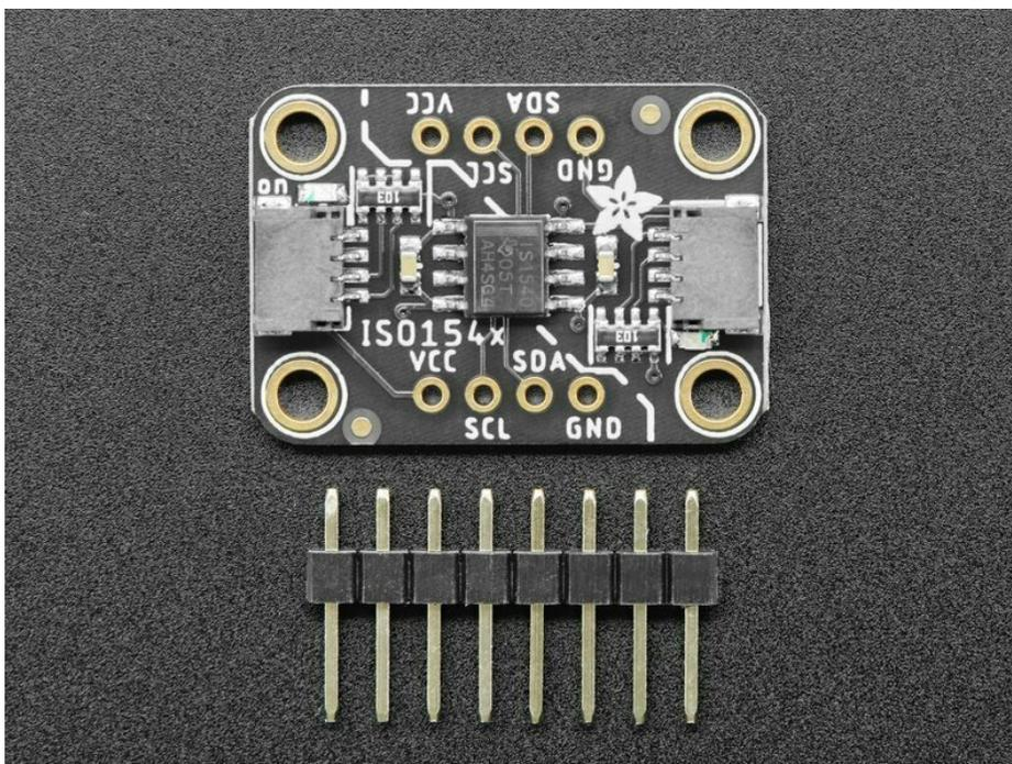
Whatever it is, you can use the **Adafruit ISO1540 Bidirectional I2C Isolator** to add full electrical isolation between two sides of an I2C bus. The chip we use, the TI ISO1540 is fully bi-directional, supports up to 1 MHz clock rates, supports clock-stretching, works with 3 to 5V DC power or logic (separate on either side
