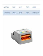
Tip: When a fault occurs, the FAULT (G22) pin will be triggered to pull down. G33 can obtain 1/10 of the input voltage and can be used to detect the current power input.
