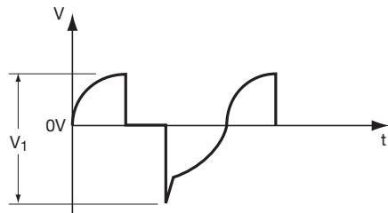
Choice of voltage:  $V_1 \leq V_{\text{peak}}$
