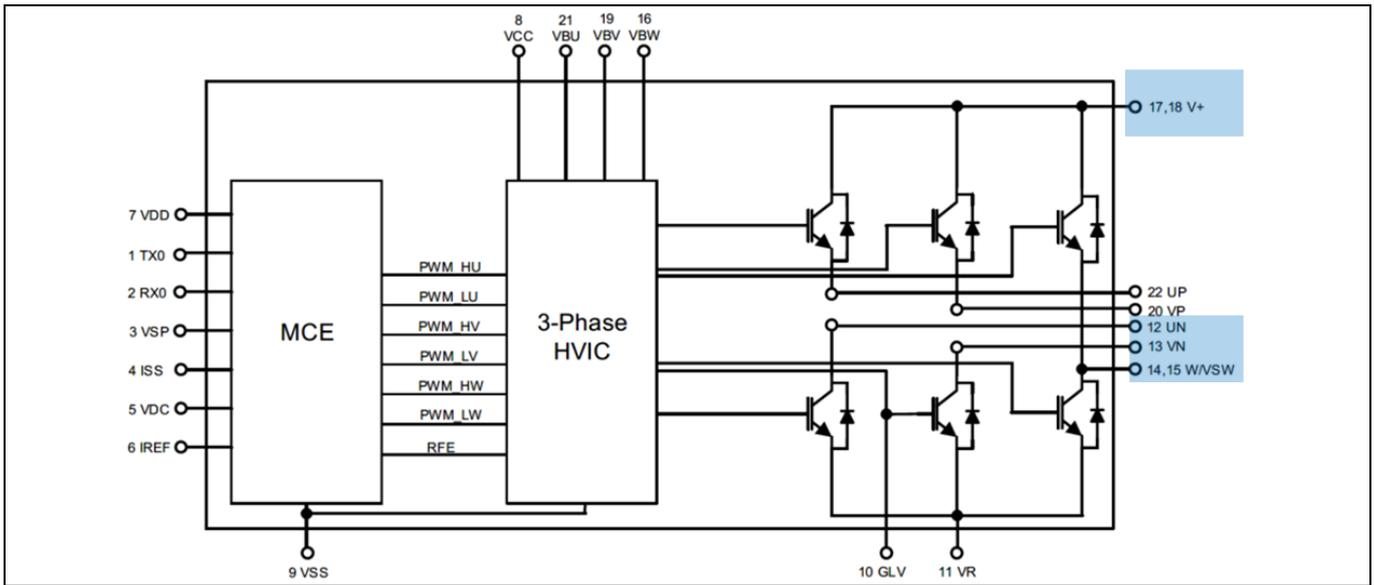
Figure 16 Critical pins for thermal PCB design
