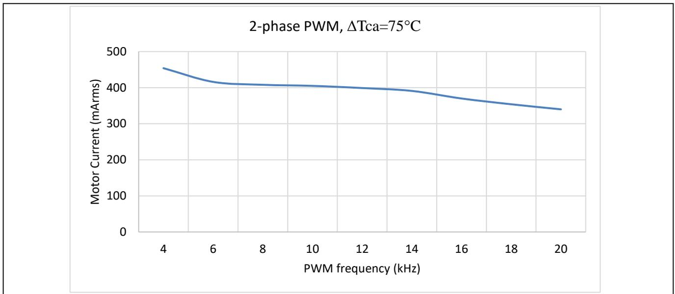
Figure 13 Thermal Characterization of IMI111T-026H, 2-phase PWM, ΔTca = 75°C, FR4 PCB with 1 oz copper
