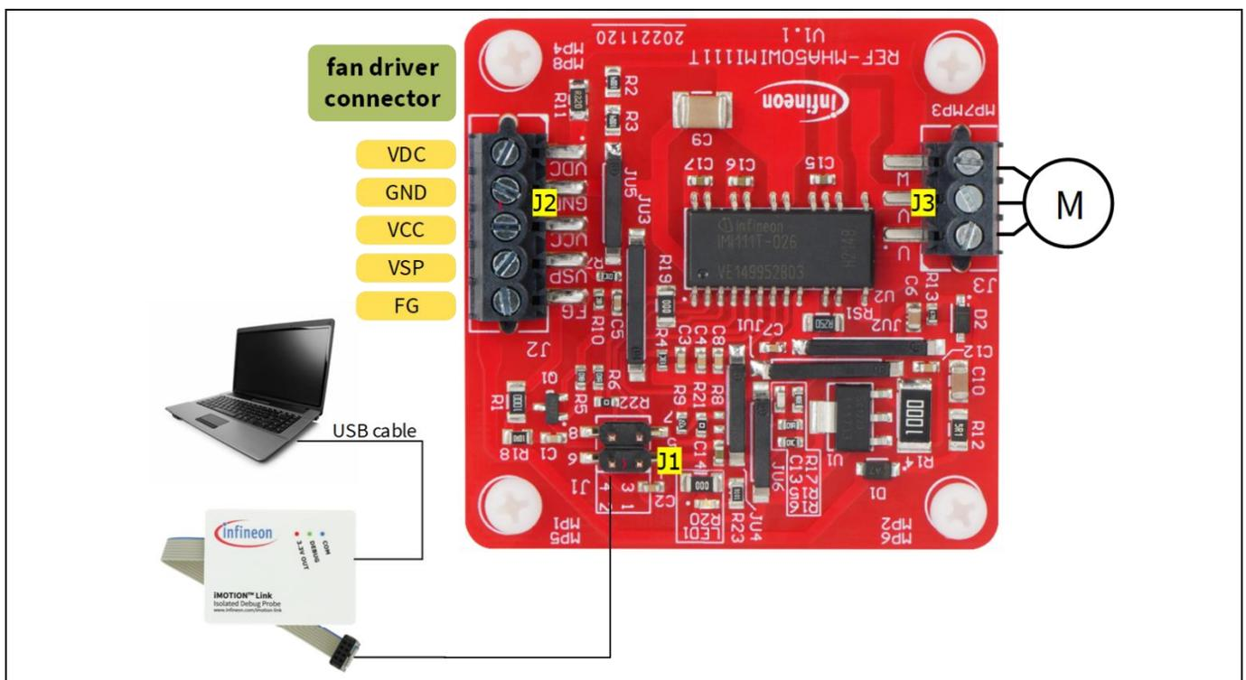
Figure 19 Using an external debugger iMOTION™ Link
