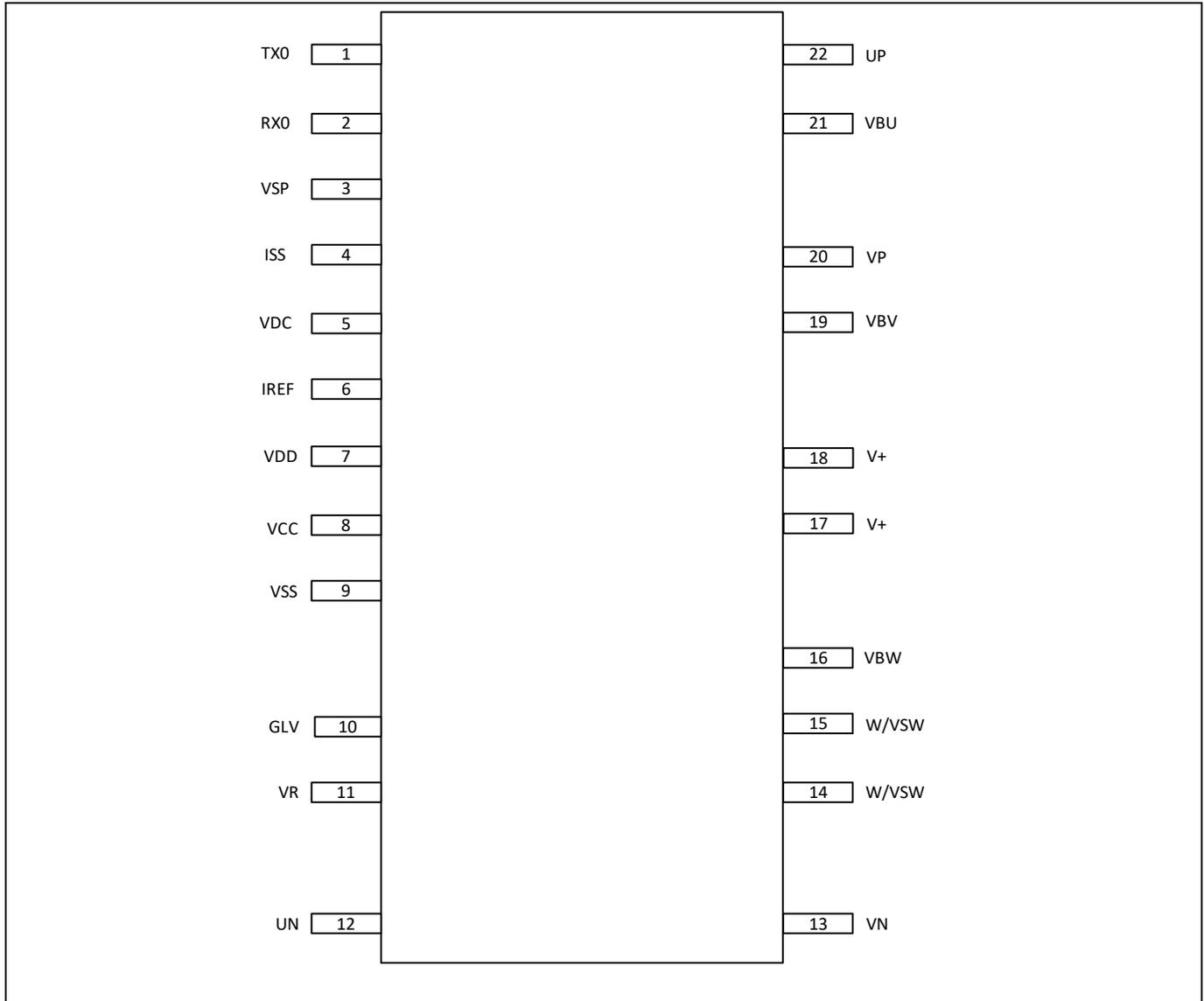
Figure 3 IMI111T pinout
