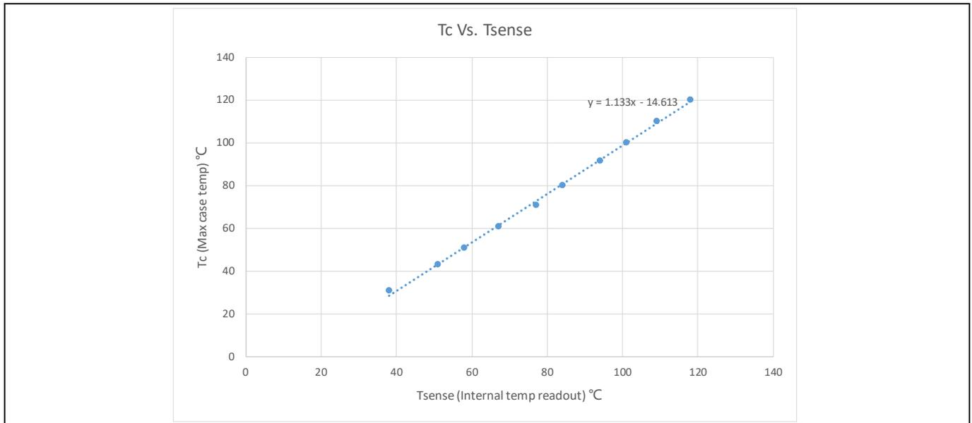
Figure 18 Correlation between the case temperature and the internal temperature readout
