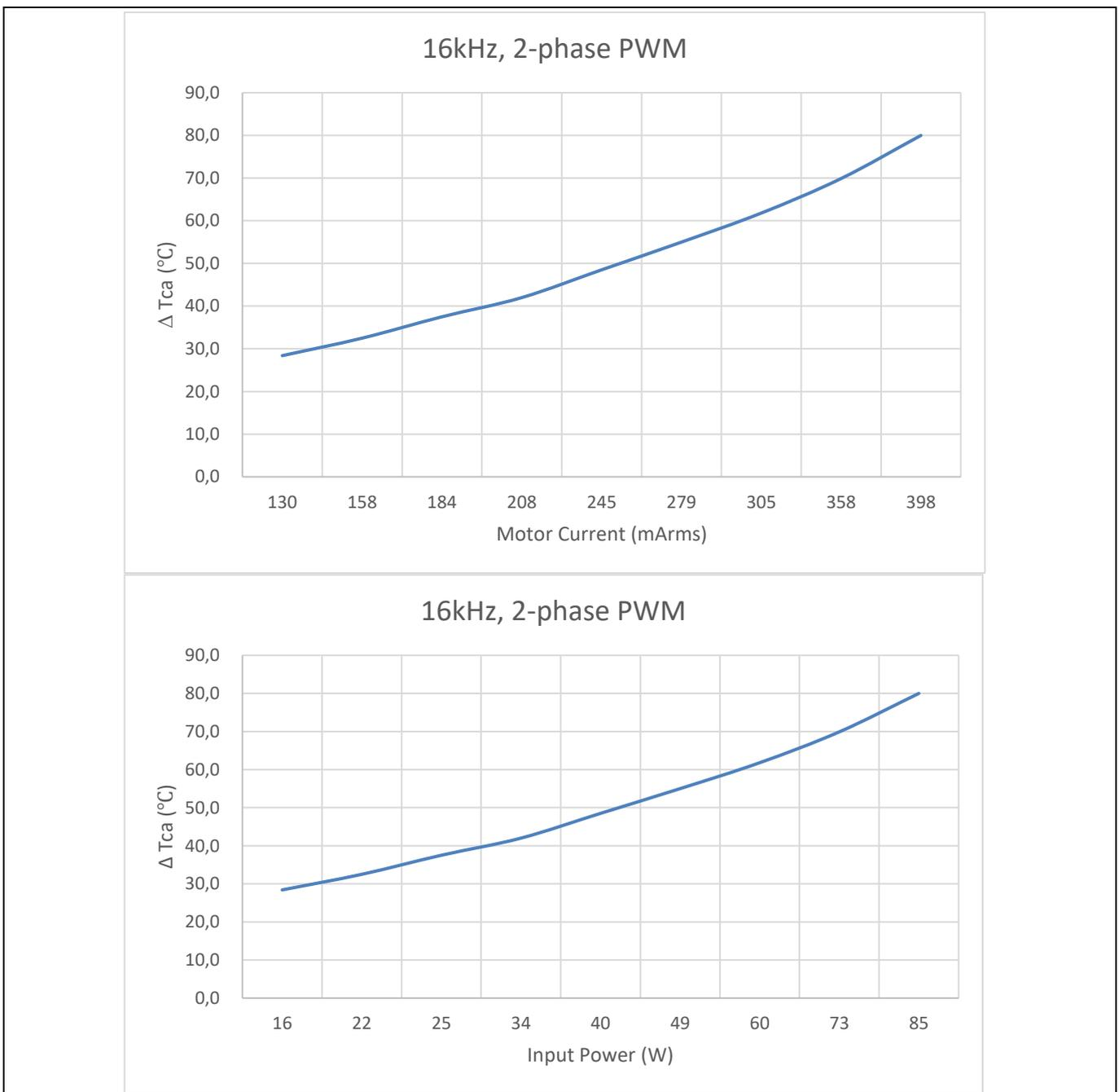
Figure 9 Thermal characterization of IMI111T-026H, 2-phase PWM, 16 kHz, FR4 PCB with 1 oz copper
