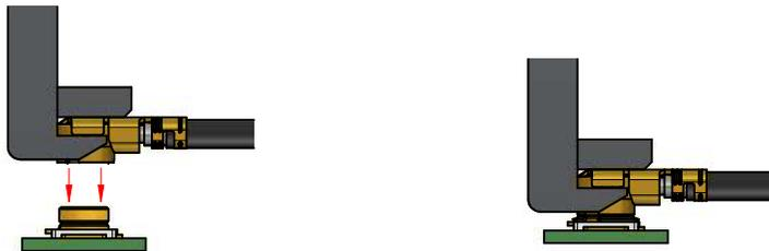
• How to unmate the UMRF plug from the receptacle ?
