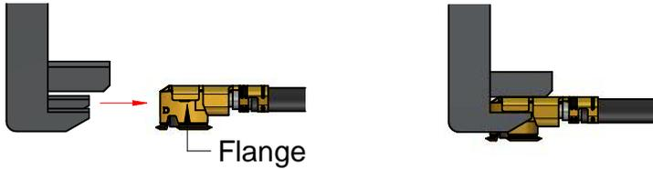
2. Align the plug to mating axes of the receptacle, and insert vertically until "click" heard to complete mated connection (Note 1)
