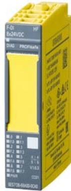
SIMATIC DP, Electronics module for ET 200SP, F-DI 8x 24 V DC HF, 15 mm width, up to PL E (ISO 13849-1)/ SIL3 (IEC 61508)
