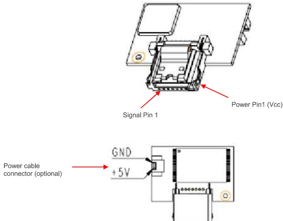
Figure 2-1 Pin Assignments – Without Housing
