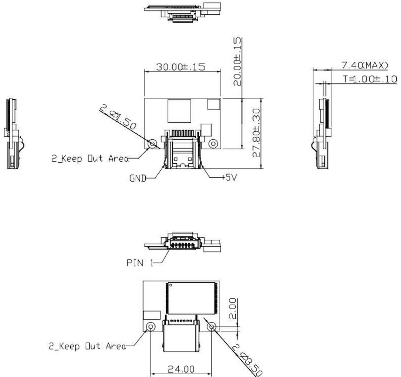
Figure 7-3 High-speed Dimensions – without Housing
