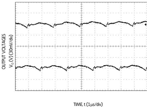
Figure 3. Typical output ripple and noise ( $C_0 = 2 \times 0.1\mu F + 2 \times 47\mu F$  ceramic,  $V_{IN} = 12V$ ,  $I_o = I_{o1,max}, I_{o2,max}$ ).
