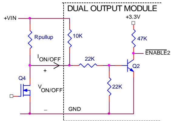
Figure 39. Circuit configuration for using positive On/Off logic.
