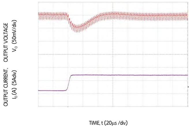
**Figure 22. Transient Response to Dynamic Load Change on one output from 50% to 100% at 12Vin,  $C_{out} = 3x47\mu F + 2x330\mu F$ ,  $C_{Tune} = 1500pF$  &  $R_{Tune} = 300$**
