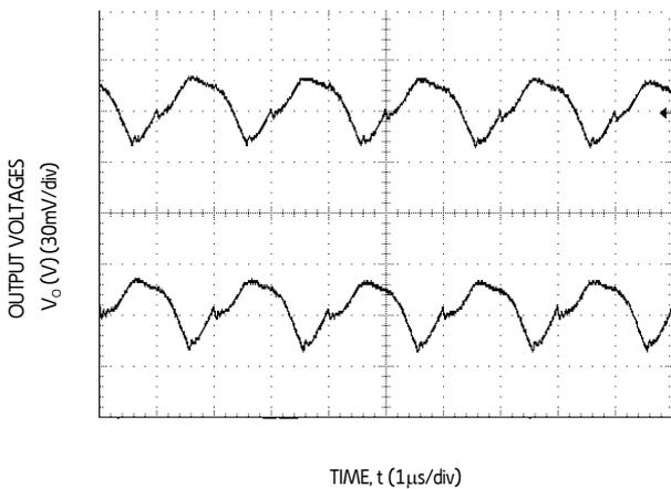
**Figure 21. Typical output ripple and noise ( $C_o = 2x0.1\mu F + 2x47\mu F$  ceramic,  $V_{IN} = 12V$ ,  $I_o = I_{o1,max}, I_{o2,max}$ ).**
