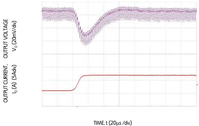
Figure 16. Transient Response to Dynamic Load Change on one output from 50% to 100% at 12Vin,  $C_{out} = 3 \times 47\mu\text{F} + 2 \times 330\mu\text{F}$ ,  $C_{Tune} = 1800\text{pF}$  &  $R_{Tune} = 300$
