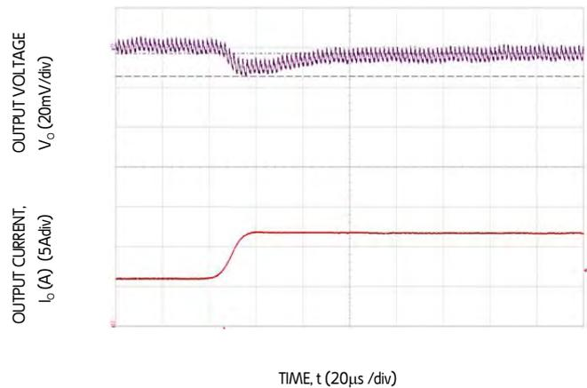
Figure 4. Transient Response to Dynamic Load Change from 50% to 100% on one output at 12Vin,  $C_{out} = 2 \times 47\mu F + 7 \times 330\mu F$ ,  $C_{Tune} = 12nF$ ,  $R_{Tune} = 300$
