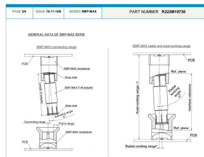
The connecting range represents the maximum misalignment during connection.
