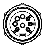
AISG 8-pin female interface with 4 loaded contacts
