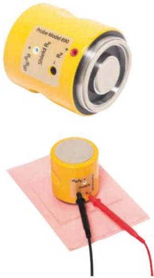
Sample application: measurement with concentric ring probe
