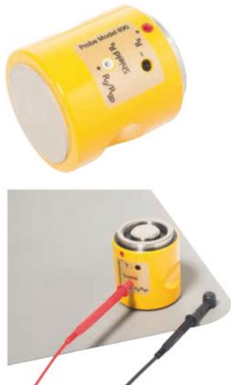
Sample application: measurement with cylindrical probe
