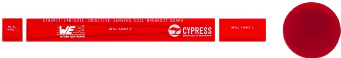
The CY8CKIT-148-COIL kit contains four metal targets, each with a different size or shape. The metal targets are meant to be broken away from the kit board and moved into the magnetic field of the desired inductive sensor.
