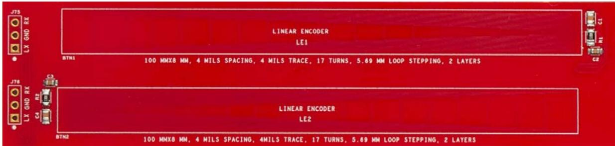
There are two 100 mm × 8 mm linear encoder coils. These coils detect horizontal movement of a METAL TARGET 2 above the sensors.
