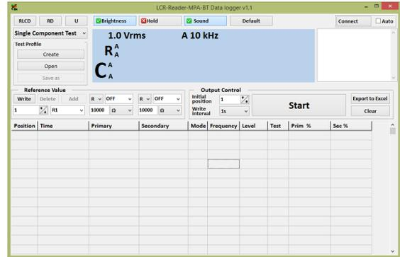
3. Connect the Bluetooth dongle and turn on **LCR-Reader-MPA-BT** and only then click '**Connect**' in the top right corner of the screen. You may need to uncheck the 'Auto' box before pressing 'Connect'.
