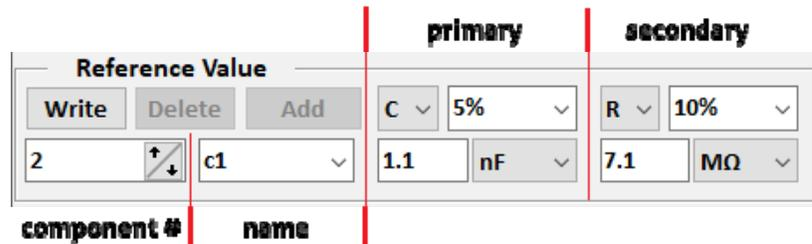
5. Now you are ready to start testing. Connect the component to the test leads and press the Space Bar on the keyboard to make a single measurement. If the component meets the specified specs, the background of the central part of the screen will be blue, otherwise it will be red. The result will also be shown in the table in the lower part of the screen, showing the measured values and '**Pass**' or '**Fail**' in the **Test** column as shown below:
