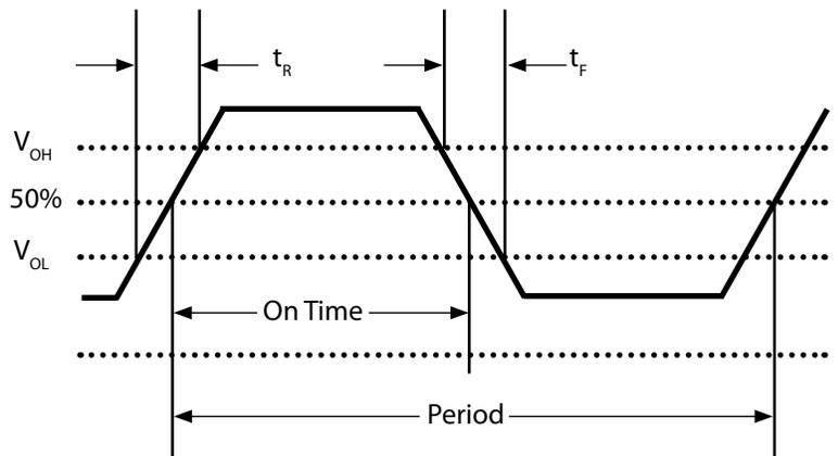
**Fig 2: LV-PECL Waveform**
