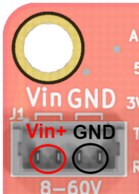
Figure 4: Voltage input header pinout
