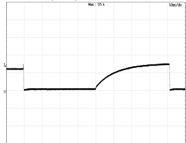
Figure 8: Output over voltage protection at 48Vin, 24A Iout CH1: VOUT, 10V/div, 50mS/div
