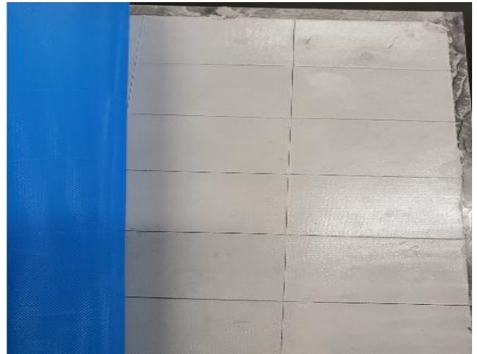
Figure 7. Replace the Blue liner on the Converted Parts after waste removal on the edge.
