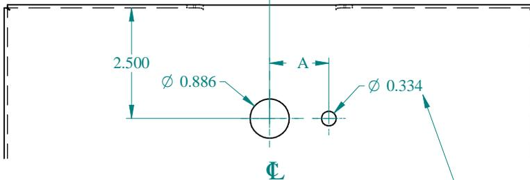
DRILLING DETAIL TOP VIEW
