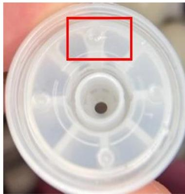
**Figure 1. Piston with fine hole defect**
