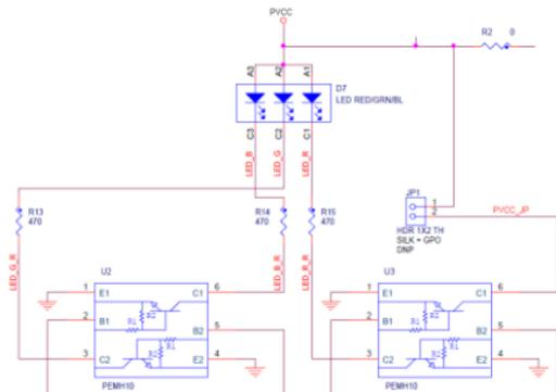
Figure 5: On-board circuit options associated with pin VCC
