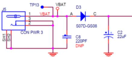
Figure 8: Power supply circuit
