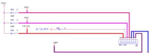
Figure 3: J3 Header (supply connector) pin mapping options
