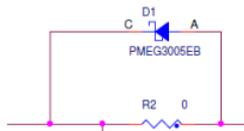
Figure 4: Reverse supply protection with D1
