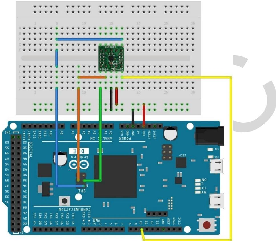
The EV3419A evaluation board can be easily wired to any microcontroller. This example shows a typical Arduino DUE platform. Please refer to the illustration below for connecting the related pins and then port the code to get the raw X, Y, Z sensor data.
