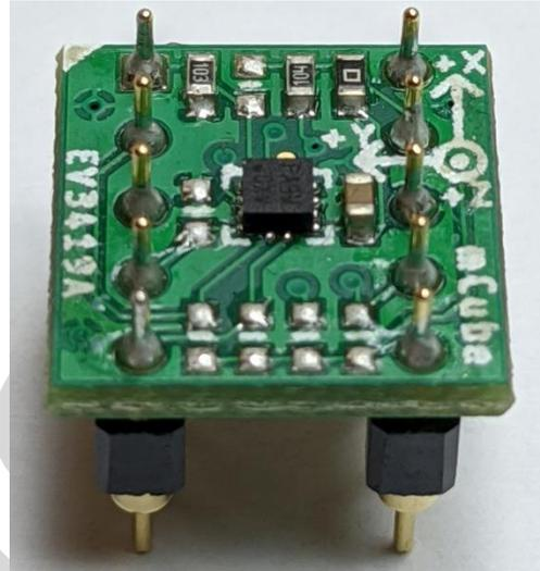
**R4, R5:** If using I2C and I2C pull-up resistors are needed for your application then install ~4.7K $\Omega$  resistors into R4 (SCL clock pin) and R5 (SDA data pin) which are not installed by factory default. In addition, besides soldering resistors on R4/R5, you can add axial lead 4.7K ohm resistors to the SDA and SCL pin respectively. It will work the same either way.
