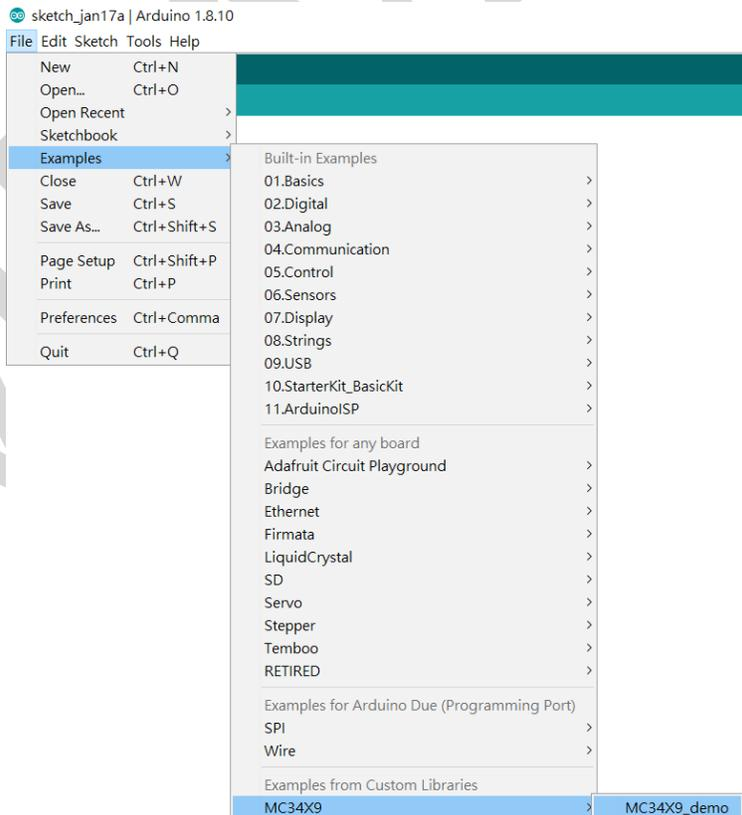
If you need the sensor running on SPI, please configure the bus as SPI in the MC34X9\_demo.ino shown as below. Otherwise, the default is I2C bus.
