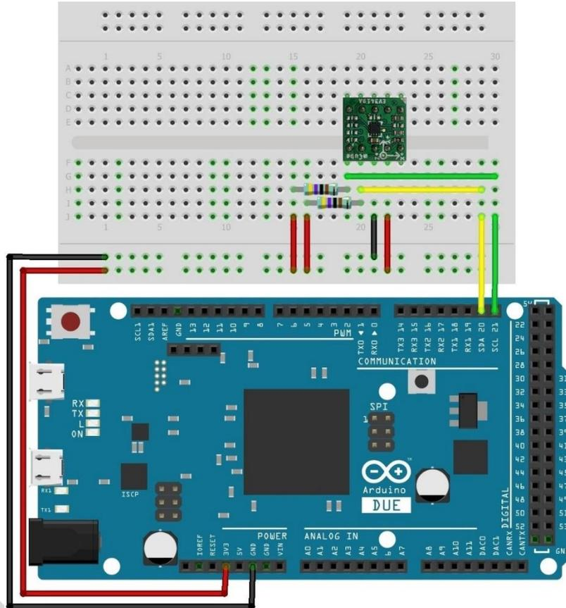
The EV3419A evaluation board can be easily wired to any microcontroller. This example shows a typical Arduino DUE platform. For other microcontrollers, be sure it has I2C with repeated-start support, then port the code. Please refer to the illustration below to connect the related pins.
