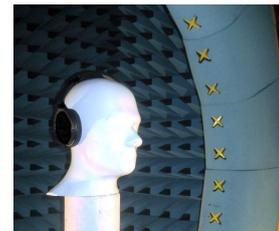
Anechoic chambers and full equipped in-house lab
