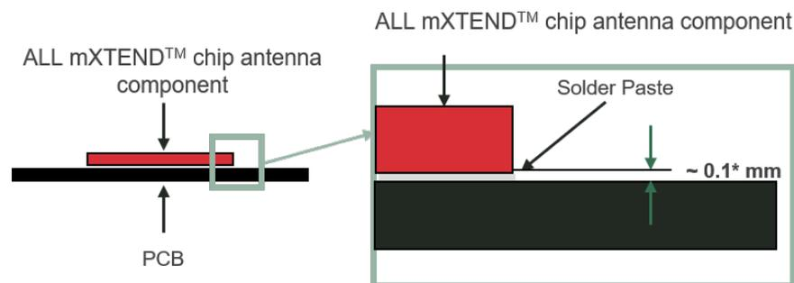
**Figure 7** – Soldering Details.
