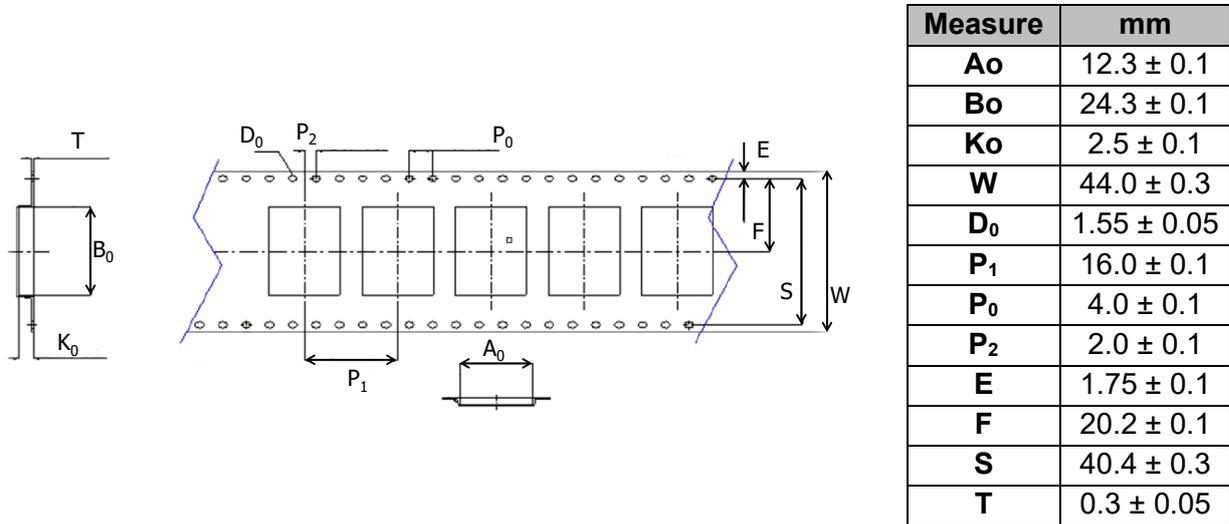
Figure 9 – Tape dimensions and Tolerances.
