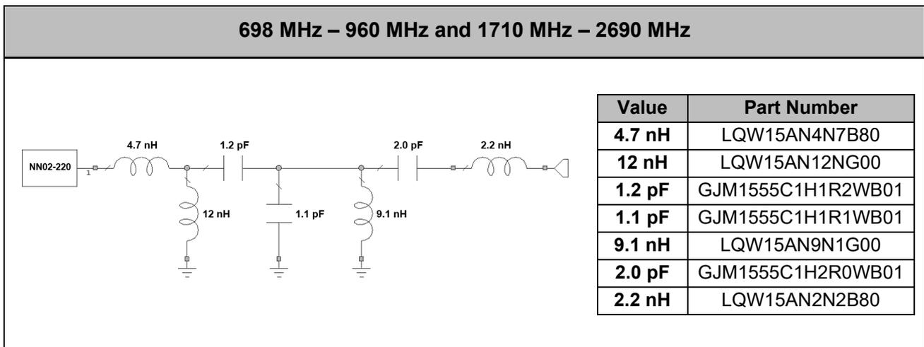
**Figure 2 – Matching network implemented in the Evaluation Board 1 port (Figure 1).**
