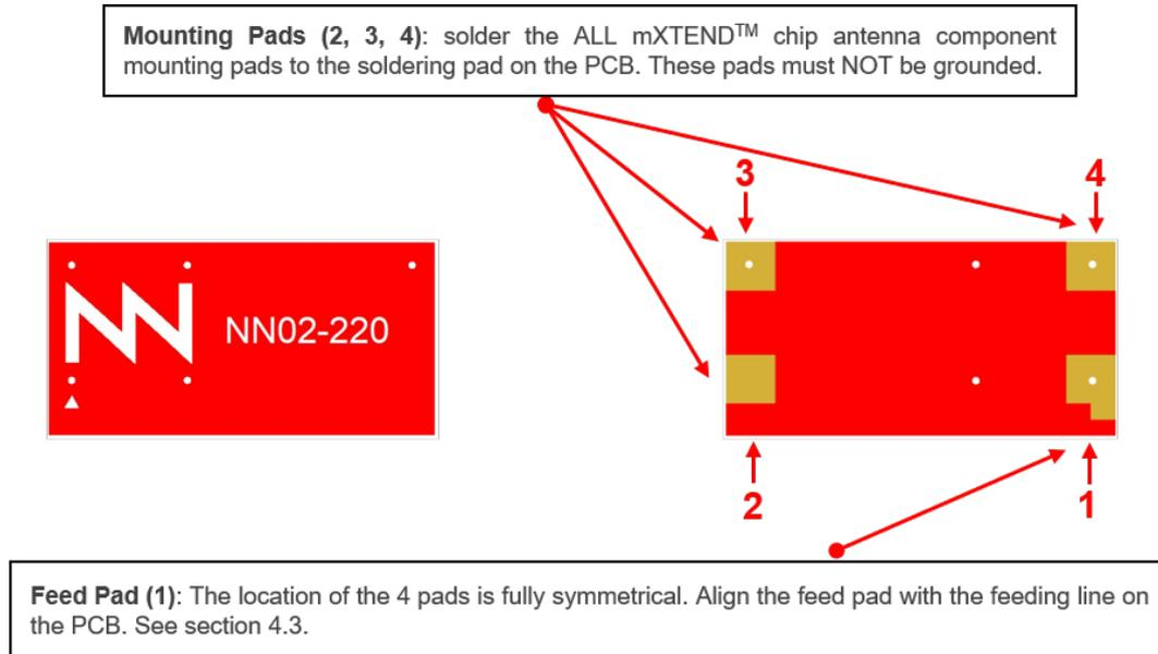
**Figure 6** – Pads of the ALL mXTEND<sup>™</sup> chip antenna component NN02-220.
