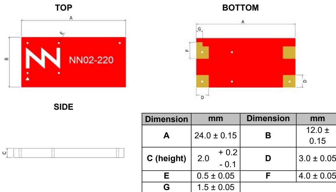
**Figure 4** – ALL mXTEND<sup>™</sup> chip antenna component dimensions and tolerances.
