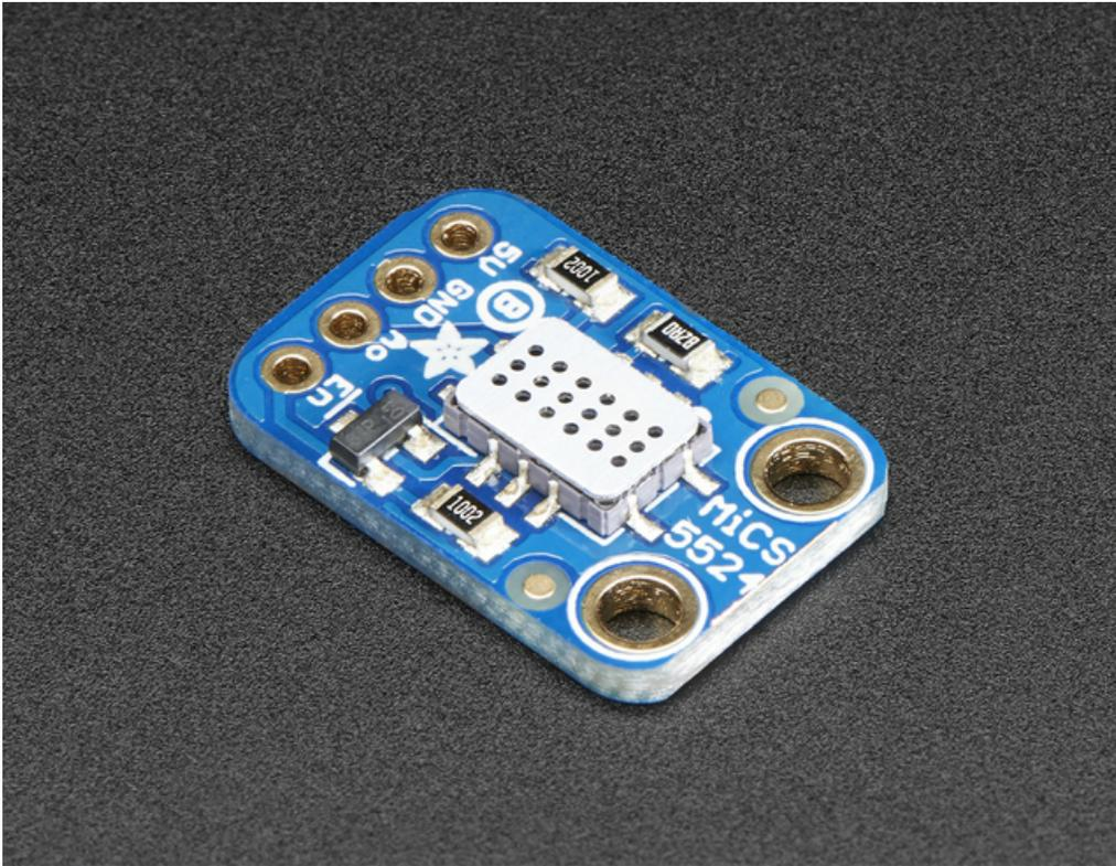
Give your next sensor project a nose for gasses with the Adafruit MiCS-5524 Gas Sensor Breakout. This breakout makes it easy to use this nice sensor from SGX Sensortech. The MiCS-5524 is a robust MEMS sensor for indoor carbon monoxide and natural gas leakage detection, it's suitable also for indoor air quality monitoring; breath checker and early fire detection.
