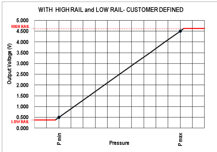
OEM Custom Calibration High/Low Rail values can be adjusted by circuit
