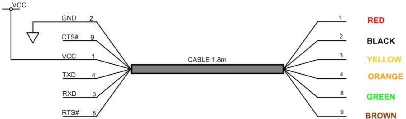
Figure 4-1 USBC-FS-UART-5V-5V-1800-WE Connections (nos. refer to pad numbers on the PCB)
