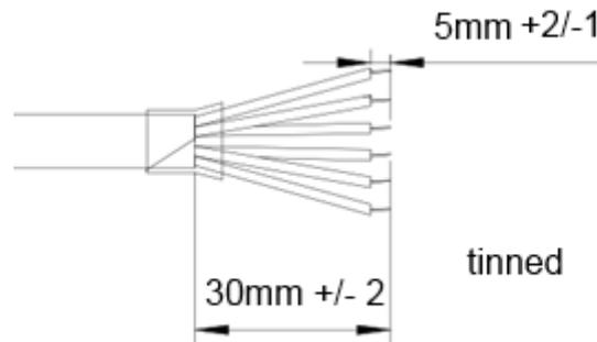
Figure 4-2 USBC-FS-UART-5V-5V-1800-WE Mechanical Details (dimensions in mm)
