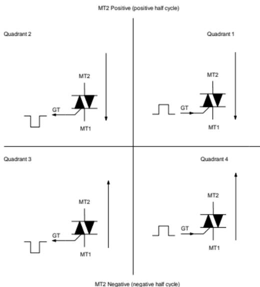
The main load current is handled by the connections MT1 and MT2. The device is switched to the on state by a current into (or out of) the gate terminal with respect to the MT1 terminal.
