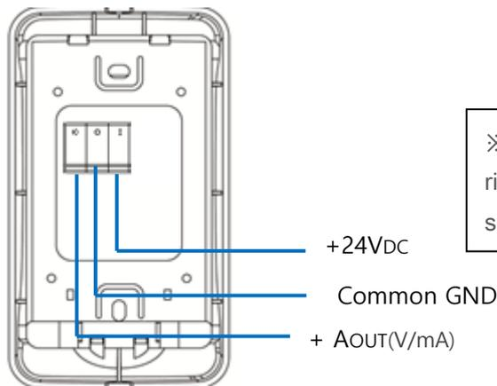
※Please make it sure to use +24VDC power wire only on right location because the insertion into wrong location such as AOUT port brings the serious failure.
