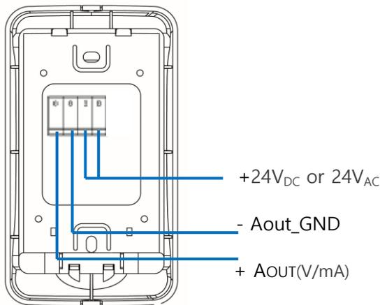
※Please make it sure to use either 24VDC+ or 24AC(+/-) power wire only on right location because the insertion into wrong location such as AOUT port brings the serious failure.
