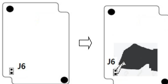
※ Locate sensor powered at fresh air where Co gas is not exist (0ppm). Let J6's two holes short, using tweezers or so, to initiate Zero-calibration takes 2~2.5 minutes until LED blinking stop.
