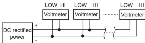
(Fig. 3) In case of using multiple voltmeter
