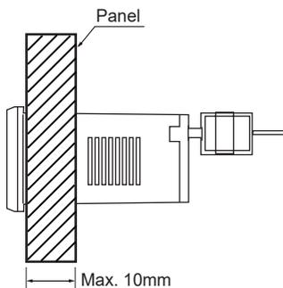
※Panel board thickness should be less than 10mm.
