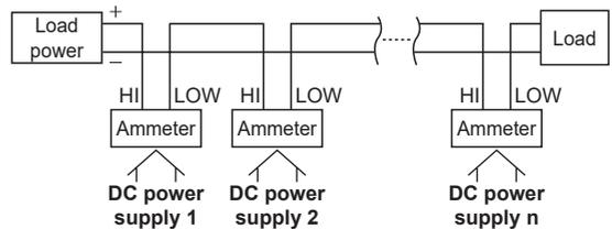
(Fig. 6) In case of using multiple ammeter
