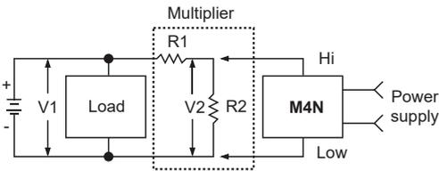
(Fig. 2) Measuring input (V1) is under 200VDC
