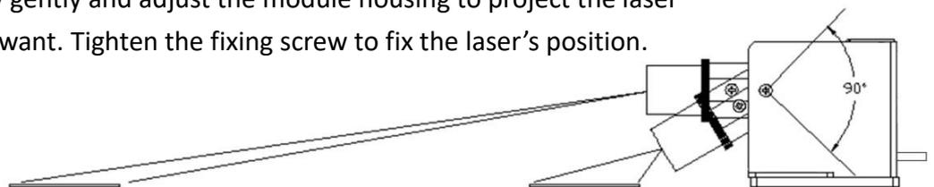
7. Loosen the fixing ring. Rotate the adjustable bushing to find the angle you want. Tighten the fixing ring to fix the laser line's angle.
