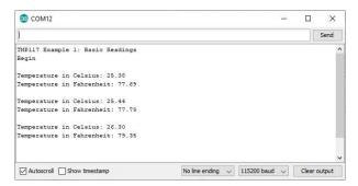
Try heating the sensor with your finger or lightly breathe some air across the sensor to watch the temperature values change! The third reading from the output shows the temperature rising after placing my finger on the temperature sensor. Remember, the sensor is taking a few readings and averaging them together before we are able see the output. Make sure to be patient with the output.
