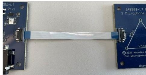
**Note:** Left side of connector is open and right side is closed to illustrate difference in the pictures.
