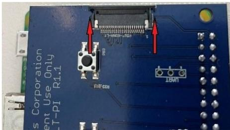
Figure 3: Open Flex Connector
