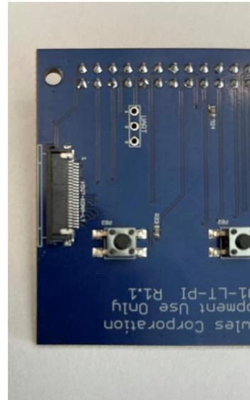
Figure 4: Closed Flex Connector
