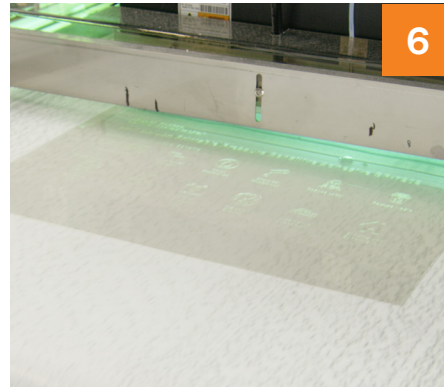
Transfer printed design to UV cure chamber.
