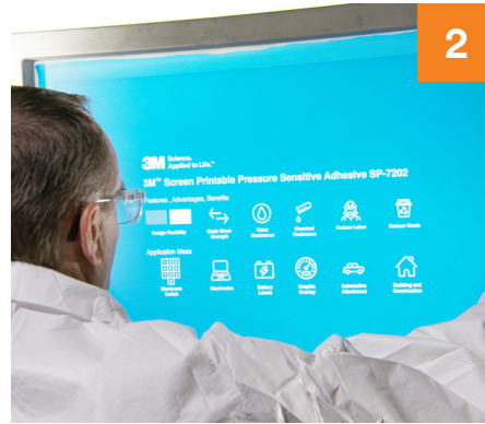
Inspect and install screen.
