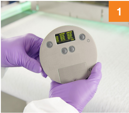
Validate UV cure chamber conditions.
