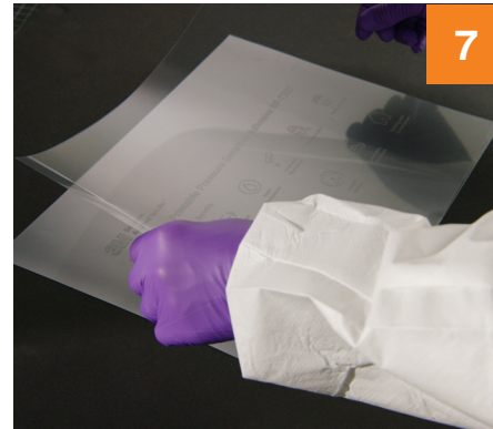
Part can be bonded immediately or a release liner can be added.
