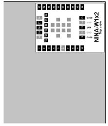
Figure 28: Placement of NINA-W1x2 with internal PIFA antenna
