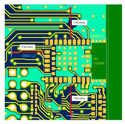
Figure 29: GND plane guard area enclosing the NINA-W1x6 module
