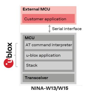
Figure 6: NINA-W13/W15u-connectXpress software structure
