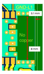
Figure 30: Size of the GND cut out for the NINA-W1x6 module's PCB trace antenna
