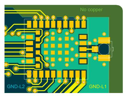
Figure 27: Example of RF trace and ground design from NINA-W1 Evaluation Kit (EVK)
