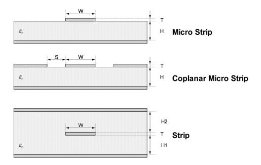
Figure 26: Transmission line trace design
