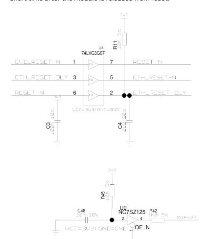
Figure 4: EVK-NINA-W1 RMII clock delay circuit
