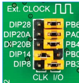
Figure 4-9: Position of the jumpers for DIP14
