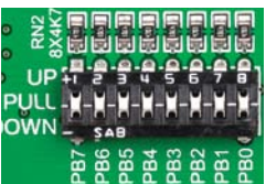
Figure 9-2: Tri-state DIP switch on PORTB
