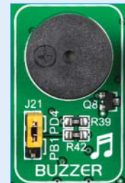
Figure 18-2: Use jumper J21 to connect Piezo buzzer on PB1 or PD4 pin
