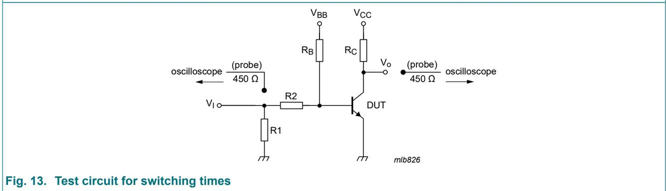
Fig. 13. Test circuit for switching times
