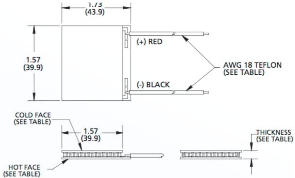
Ceramic Material: Alumina ( $Al_2O_3$ )
