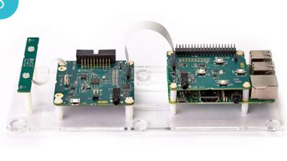
Screw longer spacers into place on top of RPi and then push Pi HAT onto RPi. Use plastic screws to fix Pi HAT board on top of the RPi.
