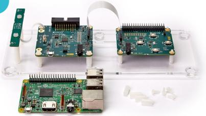
Undo plastic screws and remove large plastic spacers that hold the Pi HAT board in place. Take care not to damage the ribbon cable.
