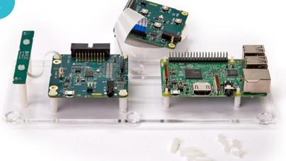
Fix Raspberry Pi to plastic stand using shorter plastic spacers to support the Raspberry Pi.
