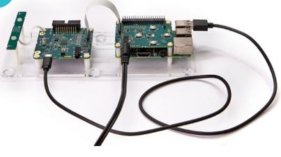
Connect speaker cable to 3.5mm LINE OUT socket on Pi HAT. Connect USB socket on XVF3510 base board to USB socket on Pi to power XVF3510.
