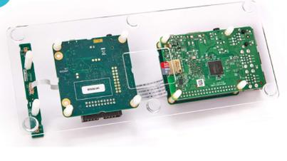
Turn kit over and slide SD card (with NOOBS installed) into Pi through the hole in kit stand.
