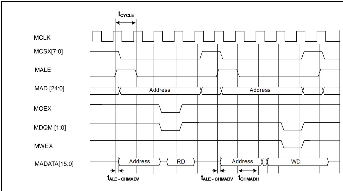
**Multiplexed Bus Access Synchronous SRAM Mode**
