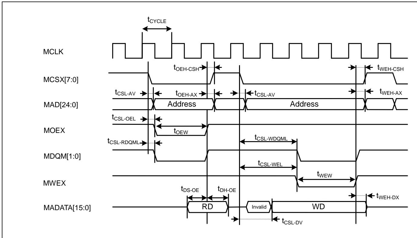
**Separate Bus Access Synchronous SRAM Mode**
