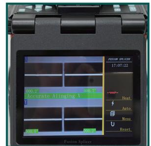
Separate X or Y axis views with 300 times magnification
