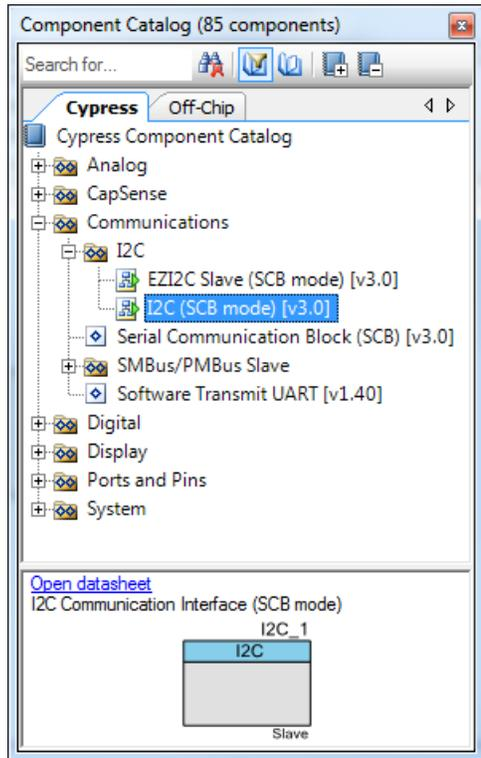
5. To configure the I<sup>2</sup>C Component, double-click or right-click the I<sup>2</sup>C Component and select **Configure**, as shown in Figure 6-5.
