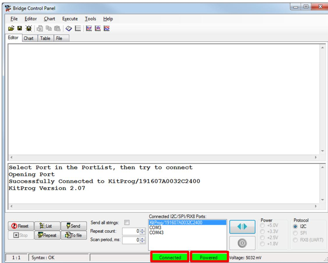
USB-I<sup>2</sup>C is implemented using the USB and I<sup>2</sup>C components of PSoC 5LP. The SCL (P12\_0) and SDA (P12\_1) lines from the PSoC 5LP are connected to the SCL (P1\_2) and SDA (P1\_3) lines of the PSoC 4 I<sup>2</sup>C. The USB-I<sup>2</sup>C bridge currently supports I<sup>2</sup>C speed of 50 kHz, 100 kHz, 400 kHz, and 1 MHz.
