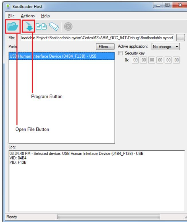
Figure 6-54. Select Bootloadable .cyacd File from Bootloader Host
