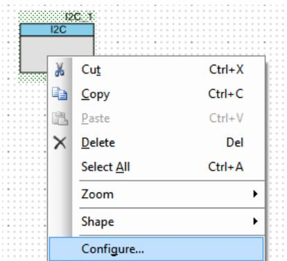
6. Configure the I<sup>2</sup>C with the settings and click **OK**, as shown in [Figure 6-6](#) and [Figure 6-7](#).
