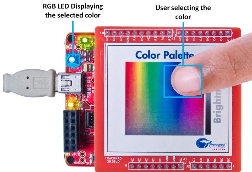
2. Move through the slider area provided at the right corner of the Trackpad to adjust the brightness level of the color. Observe the color varying from Off to full brightness from one end to other.
