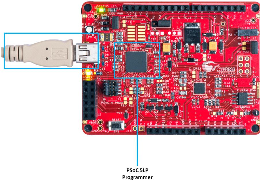
2. The onboard PSoC 5LP uses serial wire debug (SWD) to program the PSoC 4 device. See [Figure 3-5](#).
