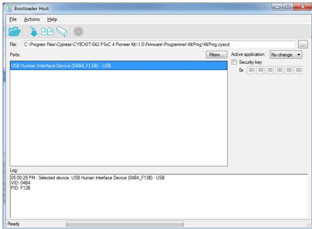
4. Click the **Program** button (or menu item **Actions > Program**) to restore the factory program by bootloading it onto the PSoC 5LP.
