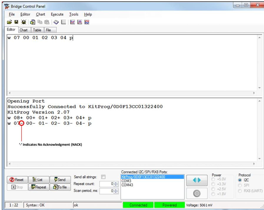
14. From the BCP, read five bytes of data from the I<sup>2</sup>C slave device with slave address 0x08, as shown in Figure 6-14. The log shows whether the transaction was successful.
