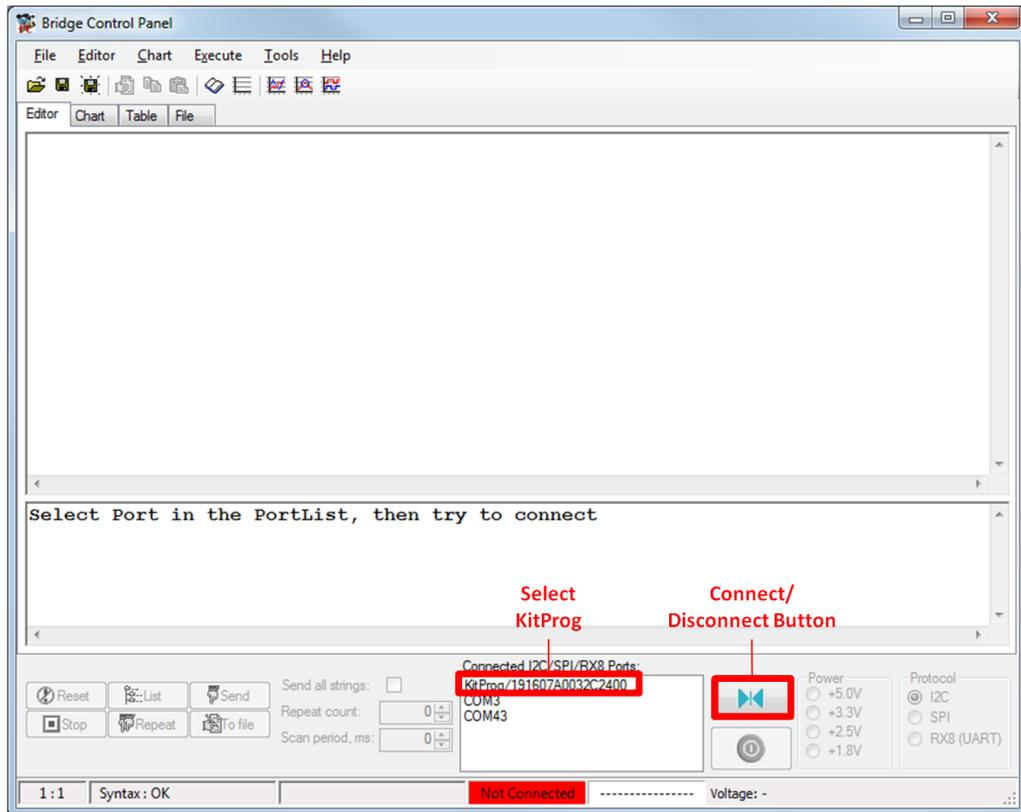
To use the USB-I<sup>2</sup>C functionality, select the **KitProg/<Serial\_Number>** in the BCP (Figure 3-10). On successful connection, the **Connected** and **Powered** status boxes turn green (Figure 3-11).
