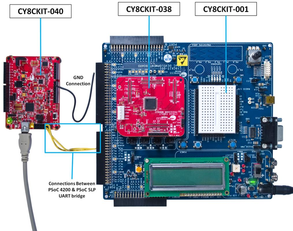
Figure 6-30. Block Diagram of UART Connection Between PSoC 4 and PSoC 5LP
