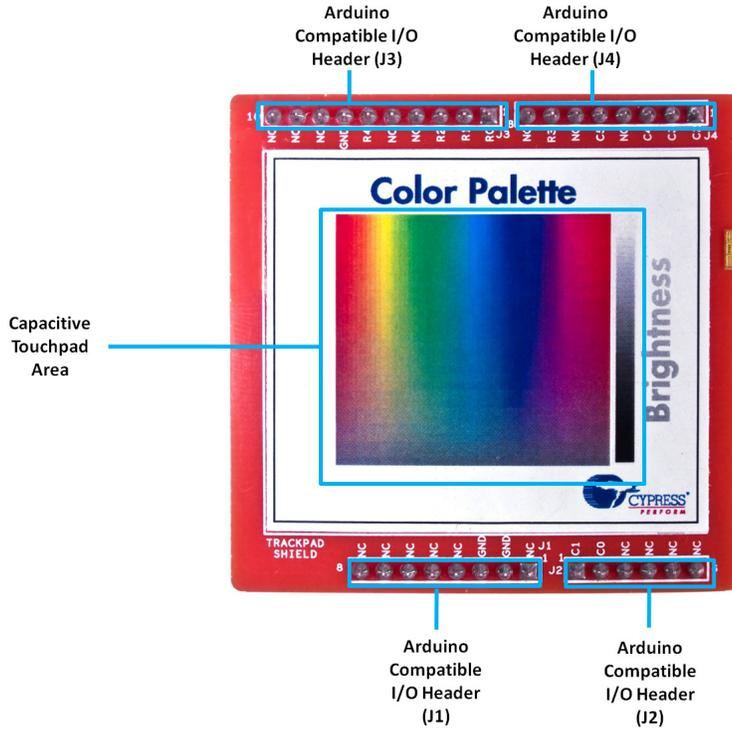
Figure 4-3. PSoC 4000 Pioneer Kit Pin Mapping
