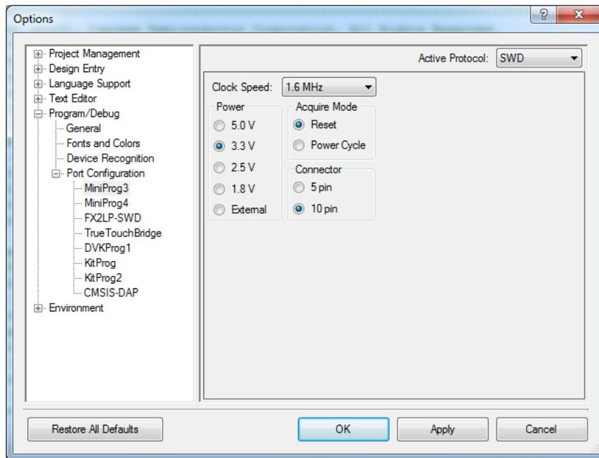
**Note:** Ensure that both MiniProg3 (with or without power) on header J6 and KitProg are not connected to the onboard PSoC 4 at the same time. This will result in failed device acquisition from both.
