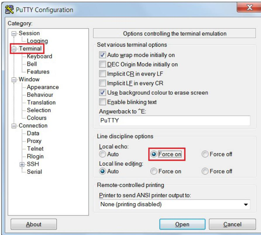
7. The COM terminal software displays both the typed data and the echoed data from the PSoC 4 UART, as shown in [Figure 6-39](#) and [Figure 6-40](#).
