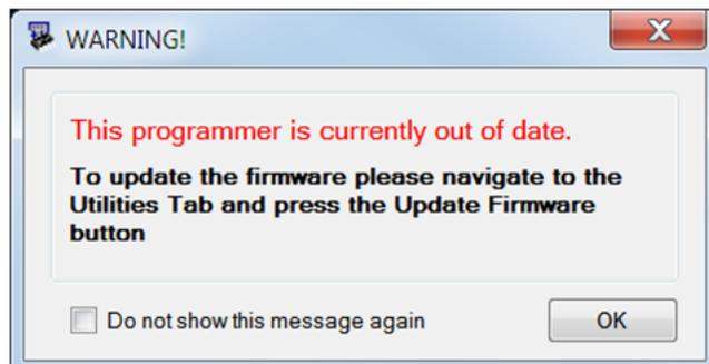
Click **OK** to close the window. On closing the warning window, the **Actions** and **Results** window displays **Please navigate to the Utilities tab and click the Upgrade Firmware button**, as shown in [Figure 3-13](#).
