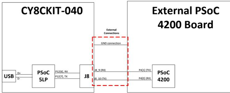
**Note:** UART RX and UART TX can be routed to any digital pin on PSoC 4 based on the configuration of the UART Component. An SCB implementation of the UART will route the RX and TX pins to either one of the following subsets: (P0[4], P0[5]) or (P3[0],P3[1]) or (P4[0],P4[1]).
