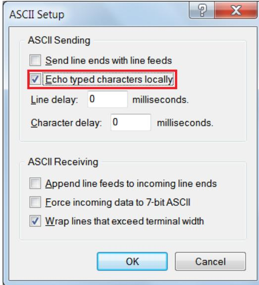
Figure 6-38. Enable Echo of Typed Characters in PuTTY
