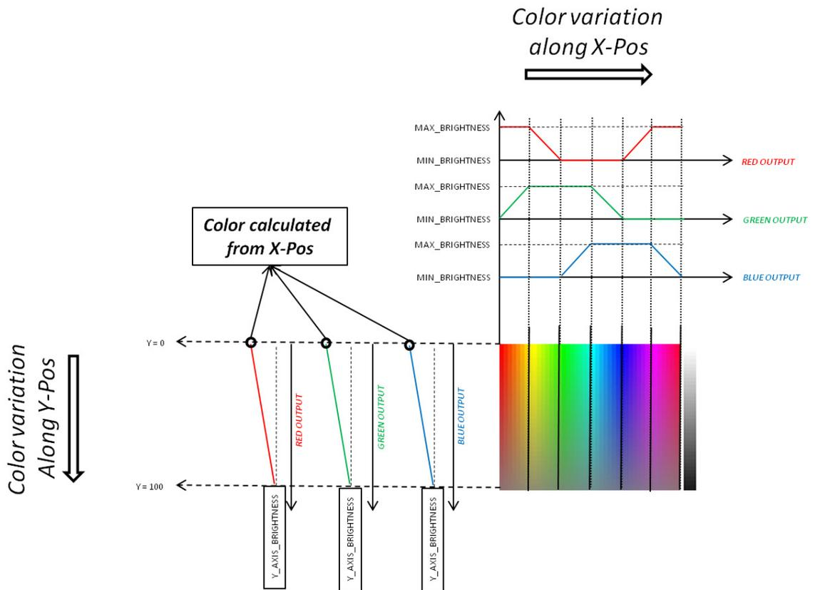
3. After the primary color intensities (from the color palette) are derived from step 2, either the brightness level or the saturation level selected by the slider is applied. The selection between brightness and saturation is done using DO\_SATURATION macro defined in *main.h*.
