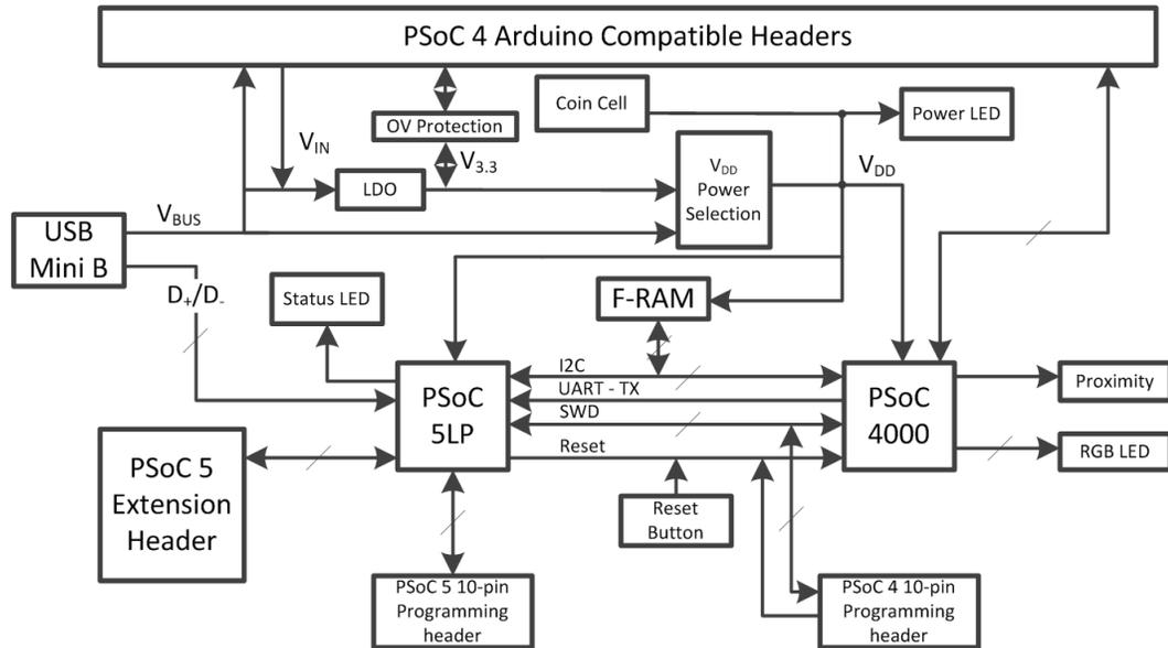
PSoC 4 is a new generation of programmable system-on-chip devices from Cypress for embedded applications. The PSoC 4000 family is the smallest member of the PSoC 4 platform with CapSense, TCPWM, I<sup>2</sup>C master or slave, and up to 20 GPIOs support. PSoC 4000 is a cost-optimized, entry-level PSoC4 device targeted as socket replacements for obsolete and/or proprietary 8-bit and 16-bit MCUs. PSoC 4000 with its ARM Cortex-M0 core brings 32 CapSense and programmable peripherals.
