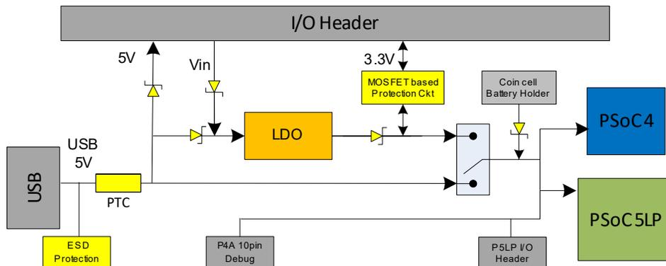
Input Voltage Range VIN is 5-12V
