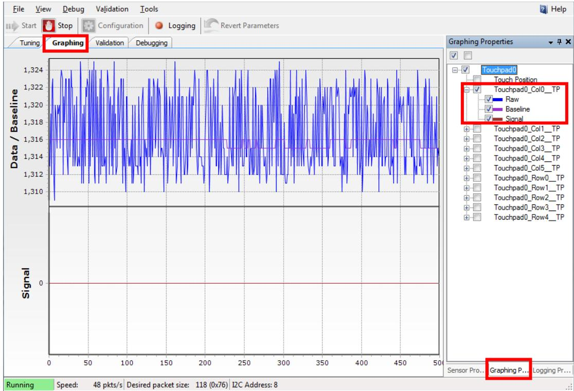
5. Touch a sensor or slider element and see the increase in Raw count and Signal, as shown in Figure 5-40.
