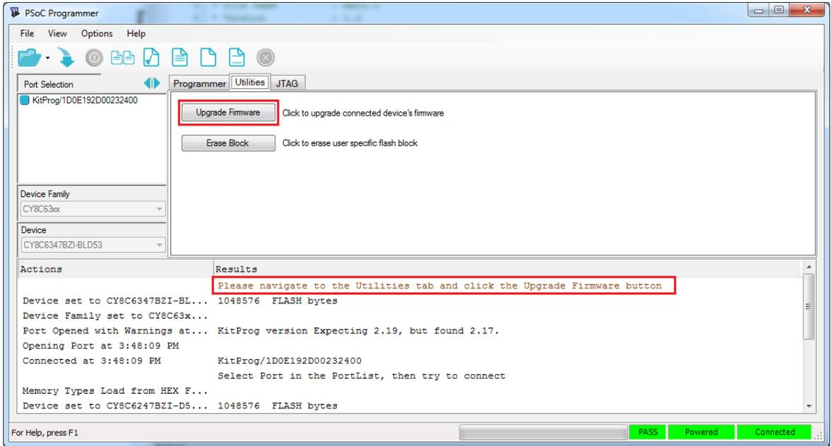
Click the **Utilities** tab and then click the **Upgrade Firmware** button. On successful upgrade, the **Actions** and **Results** window displays the firmware update message with the KitProg version, as shown in [Figure 3-14](#).
