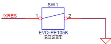
**Note:** The PSoC 4 Reset pin (XRES) has an internal pull-up resistor. However, an external pull-up resistor R10 and capacitor C30 are connected to the PSoC 4 Reset pin on the kit, which is optional and required only in a noisy system.
