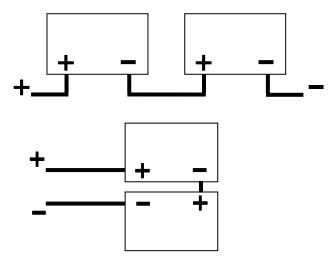
Figure 5: Possible Series Connection Arrangements
