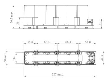
Figure 3: BMOD0058 Mounting Hole Locations
