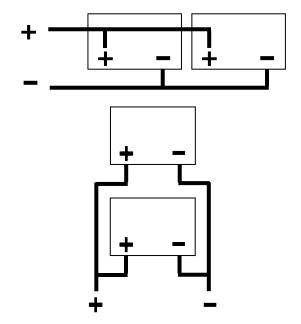
Figure 6: Possible Parallel Connection Arrangements
