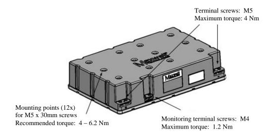
Figure 2: BMOD0006 Mechanical Configuration
