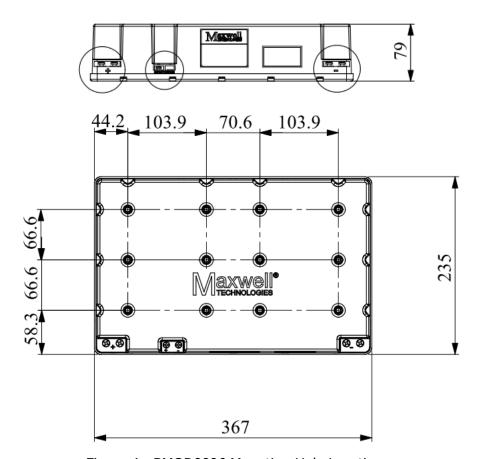
Figure 4: BMOD0006 Mounting Hole Locations
